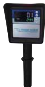
PLASTOMETER with a combined display PRESSURE / TEMPERATURE
